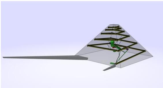
The external ramp has almost disappeared, the internal ramp is close to the top, and the last few meters will be built using a vertical shaft and a hoisting machine.
