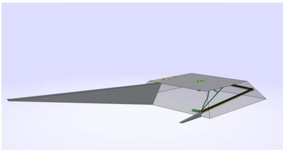
The external ramp reaches its maximum level, the internal ramp, the 3<sup>rd</sup> section of which reaches the South/West corner; due to its geometry, it does not interfere with the building site's supply. The ceilings beams of the King's Chamber are hoisted to this level with the help of the counterweight circulating in the Grand Gallery.
