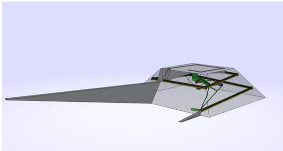
Construction of the King's Chamber has been completed, and the trench ramp extending the external ramp has reached the +70m level; it can no longer travel any further up the body of the pyramid. A large part of the storage area on the South face has been filled in, and most of the 4<sup>th</sup> horizontal section of the internal ramp has been built. The 7<sup>th</sup> section runs beneath the West face.
