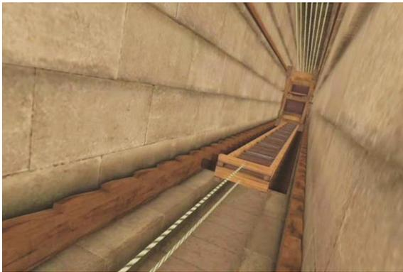
The granite beams forming the King's Chamber are hoisted up by means of the counterweights circulating in the Grand Gallery and installed permanently in each of the ceilings. Ceiling by ceiling, the King's Chamber was built with the help of the counterweight, considerably reducing the number of workers required.
