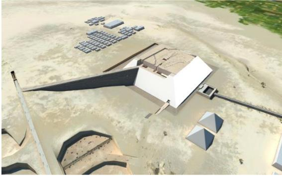
Aspect of the building site and external ramp at the time of construction of the King's Chamber
