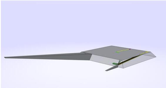
The external ramp rises at the same time as the pyramid, reaching the level of the Queen's Chamber. The 1<sup>st</sup> section of the internal ramp opens at this level in the North/East corner. The 1<sup>st</sup> rotation room is about to be built.
