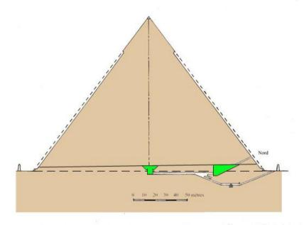
In the section shown above, we see that the funeral chamber was constructed in a, openly excavated ditch (in green, centre) before being covered by a roof made of limestone beams laid as rafters.
