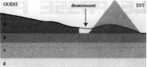
The pyramids of Khufu and Khafre were therefore built on two mounds that would have allowed a 40% saving in volume for each of them. Nothing on the site at Giza or in the pyramids supports such an assertion, and even less so at Maidum and Dahshur (Rhomboidal and Red) where the pyramids are built on flat ground. Taking this argument further, the Sphinx would have therefore been sculpted in a mound at the foot of the plateau.
