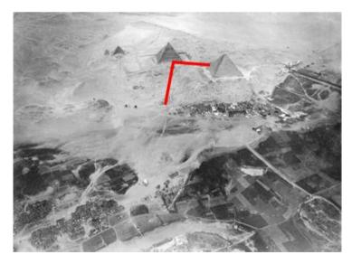
According to the theory, the exterior ramp of Khufu giving access to the construction site up to level +43 m sets out from the north-east corner of the future pyramid of Khafre and joins the pyramid in the south-east corner of its southern face.
