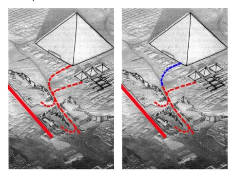
The new access path arrives slightly higher on the plateau, so about 1 m above the level of the base of the pyramid. The small ramp constructed in continuation, to reach the level of the entrance to the interior ramp, is thus reduced, there being less difference in level.
