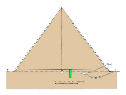
The trench, shown in green on the diagram, intersects the north-south axis perpendicularly and its position is established by the "constructed", or stone-built, section between the two "excavated" parts of this corridor.
