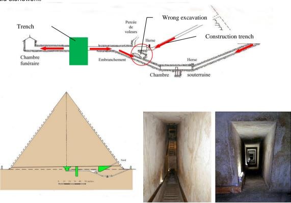
On the left: either side of the existing trench, we see the ditch excavated to create the funeral chamber and the trench excavated to construct the upper descending corridor. By analysing this section, it is clear that there was no reason to dig a new trench cutting through the horizontal corridor; on the contrary, the architects adapted their approach to this existing constraint. In the centre: the ascending corridor seen from the upper horizontal corridor.
