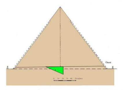
The designers considered it preferable to run the trench as close as possible to the bedrock in order to reduce the underpinning requirement as far as possible; to do this, they offset the corridor 23 cubits to the east. In addition, the trench certainly having been filled in quickly towards the end of the construction of the pyramid of Khufu, it was not necessary to completely excavate it if it was not in line with the future upper horizontal corridor.
