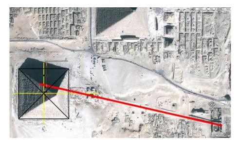
The axis of the ramp under the Royal Causeway of Khafre intersects the upper horizontal corridor of the pyramid of Khafre at a little less than one third of the distance, measured from the east-west axis, between this axis and the northern base.
