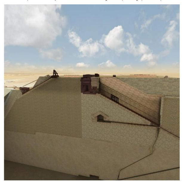
The counterweight system (on the right in this illustration), namely the platform for the beams, the set of rollers, lateral notched wooden bars, etc. as well as stones for the banks in this section, will be used first. Everything was used and reused as much as possible.
