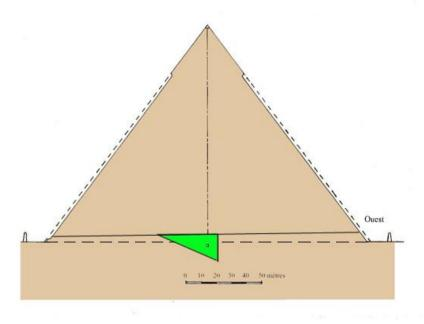
If the corridor had been positioned in the north-south axis, it would have crossed the trench where it was very deep, requiring a fairly large foundation block to be recreated, a "prop" about ten metres high, in order to find support on the rock.
