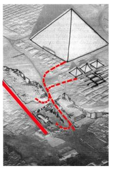
In parallel with the first ramp for the construction site of the pyramid of Khufu under the future Royal Causeway of Khafre, a third ramp joined the port and the northern quarries to the entrance to the interior ramp assumed to be located at the south-east corner of the pyramid of Khufu. The difference in level between the port and the base of the pyramid is 40 m and the route measures about 550 m, making an average slope of 7.2%.
