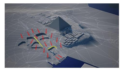
The red arrows indicate the new course of run-off water following the construction of the Khufu pyramid. The yellow lines show the first rain erosion on the quarry walls (erosion that can be seen today in the Sphinx pit and in the quarry south of the port ramp).
