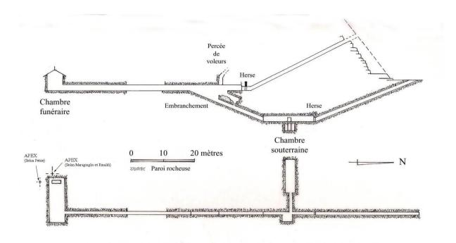
Section and plan of funeral apartments of Khafre. The horizontal corridor leading to the funeral chamber contains an anomaly: part of it is constructed and not excavated.
