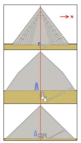
Convention during this period dictated that royal burial chambers should lie to the south of the pyramid's east/west axis. As shown in the illustration, the burial chambers in the Meidum, Bent, and Red Pyramids are all constructed south of the east/west axis, opposite the entrance. In Khufu's pyramid the King's and Subterranean Chambers both lie to the south, and the Queen's Chamber straddles the east/west axis perfectly.
