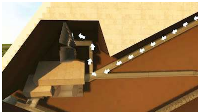
Worker's exit route
